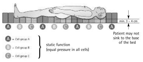
2. The cycle time on the power unit can be varied from 5 to 20 minutes. By pressing button 3 ("Cycle"), cycle time can be changed from standard 5 minutes with equal steps of 5 minutes to a maximum of 20 minutes. Within a cycle all three cell groups are inflated and deflated once.
